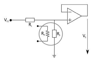
Figure 1: Schematics of the sensor readout circuit.
