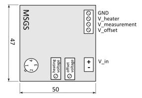
Figure 2: Schematics of the dimensions and connections of the MSGS Control Electronics
