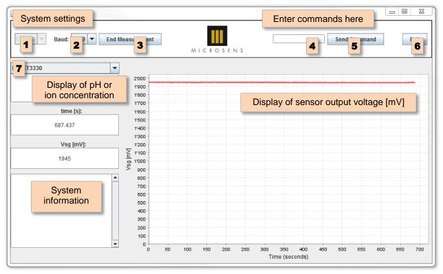
Once the measurement file is selected the graphical user interface will open, as shown in the above picture. In order to connect to the MSFET3330 Interface, the user needs to select the corresponding COM port (1). The baudrate should be set to 1200 for a correct communication between the PC and the MSFET3330 Interface (2). Clicking on "Start Measurement" (3) will start the measurement and the received data will be displayed.
